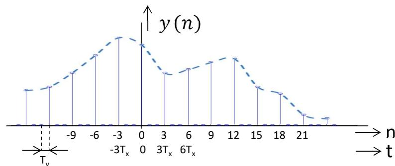
$$y(n) = \begin{cases} x\left(\frac{n}{N}\right) & \text{for } n = 0, \pm N, \pm 2N, \dots \\ 0 & \text{otherwise} \end{cases}$$
