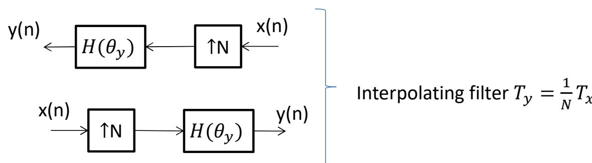
Interpolating filter  $T_y = \frac{1}{N} T_x$
