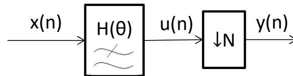
**Decimator:** Removes unwanted spectrum and induces no aliasing
