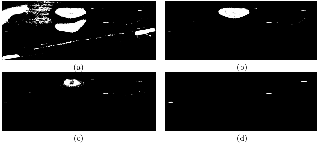
Figure 8. Input image of raindrop in camera lens (a), K-means classifier (b), Random Forest (c), U-net (d)
