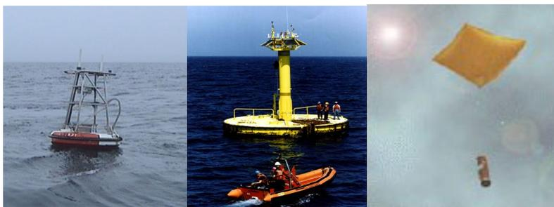
Fig. 1. Drift Buoy (left), Moored Buoy (middle), and Dropsonde (right).
