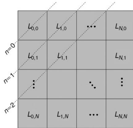
Fig. 1. A spatial representation of Hermite transform coefficients as a set of  $N \times N$  subbands  $L_{n,m}$ . The subband size depends on the subsampling factor used in the expansion. Diagonals depict zero-order coefficients ( $n = 0$ ), first-order coefficients ( $n = 1$ ), etc.
